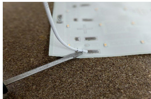
Figure 5 – Removing a wire from an IDC connector
