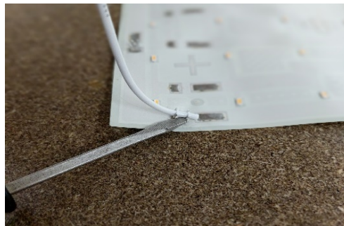
Figure 5 – Removing a wire from an IDC connector
